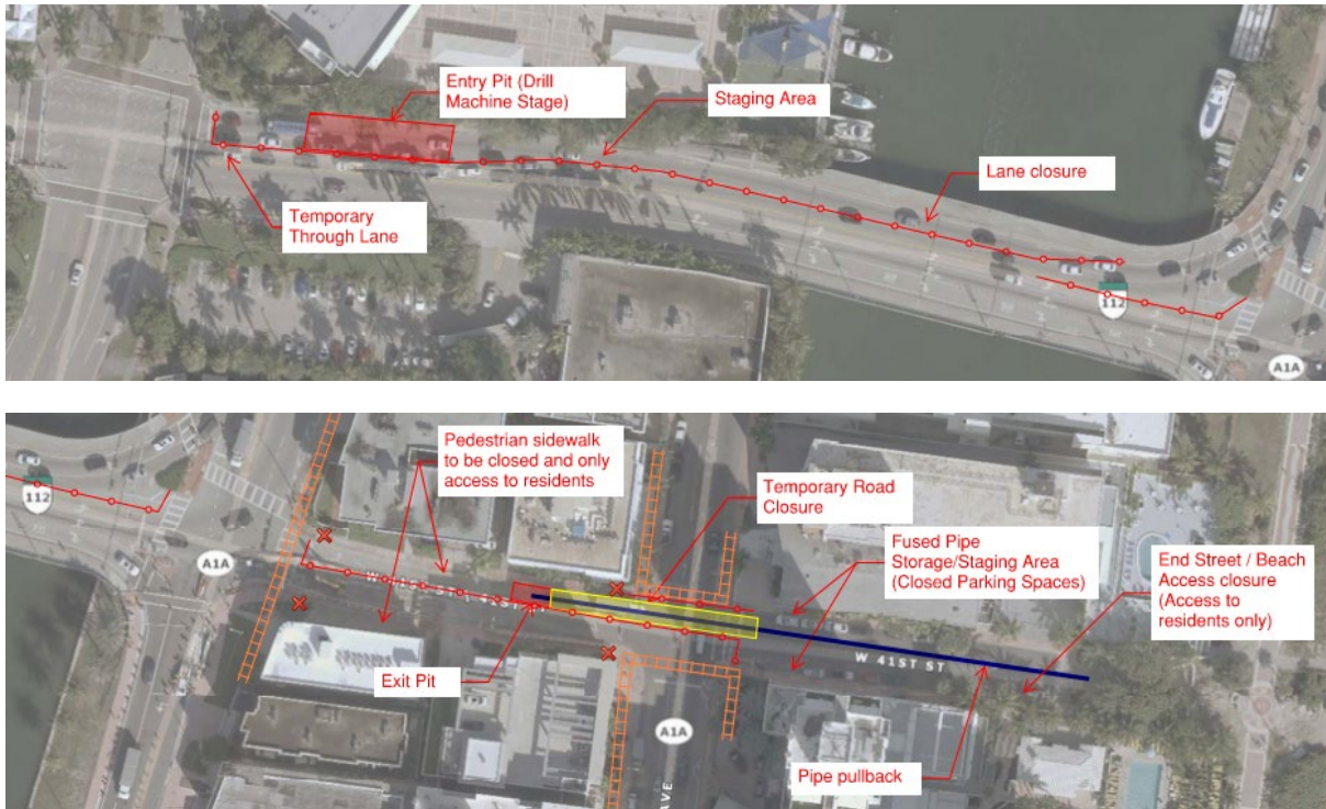
Figure 16. MOT Phase 2 – HDD Pulling
