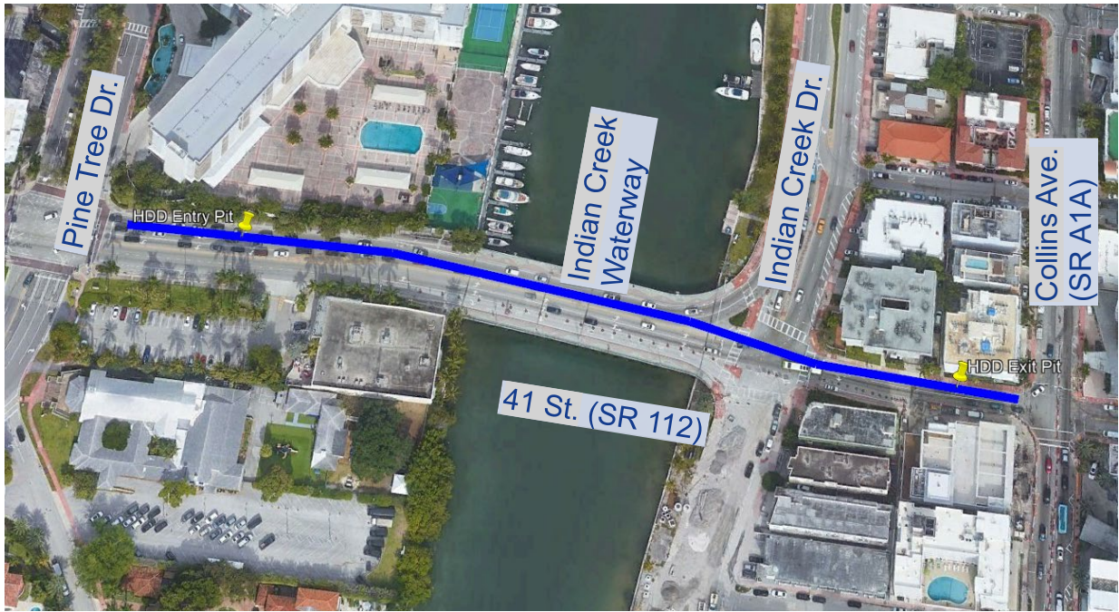
Figure 7. Proposed Water Main Horizontal Alignment
